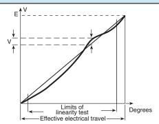
The independent linearity (conformity for the non linear laws) is the maximum gap  $\Delta V$  between the actual variation curve and the theorical variation curve the nearest to it. The linearity and the conformity are expressed in percentage of the total applied voltage E
