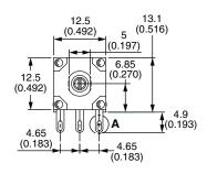
Single module, single shaft, vertical mounting, PC pins with support plate, metric bushing and shaft
