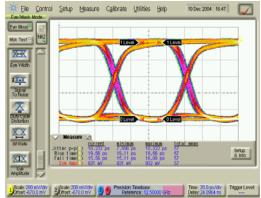
Die measurement Vee: -5.0 V Input data rate: 12.5 Gb/s Single-ended data input: +/-450 mVpp Control voltage: VCm=VFm=VCREF; VCp=-2.2 V; VFp=-3.0 V
