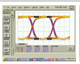
Die measurement Vee: -5.0 V Input data rate: 10.7 Gb/s Single-ended data input: +/-450 mVpp Control voltage: VCm= VFm =VCREF VCp=-2.2 V; VFp=-3.0 V
