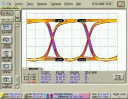
Die measurement Vee: -5.0 V Input data rate: 10.7 Gb/s Single-ended data input: +/-450 mVpp Control voltage: VCm=VFm=VCREF; VCp =-3.0 V; VFp =-3.0 V
