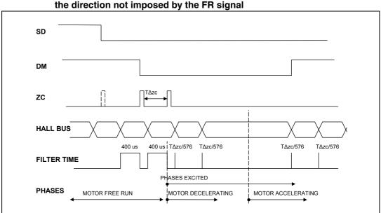
Figure 20. Startup sequence forced by SD, supposing the motor rotating quickly in the direction not imposed by the FR signal
