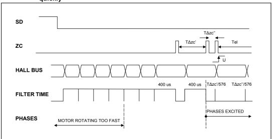
When the SD signal has a falling edge the logic waits for an Hall effect commutation. If the motor is rotating too quickly the next Hall effect commutation occurs before the filtering time has elapsed.
