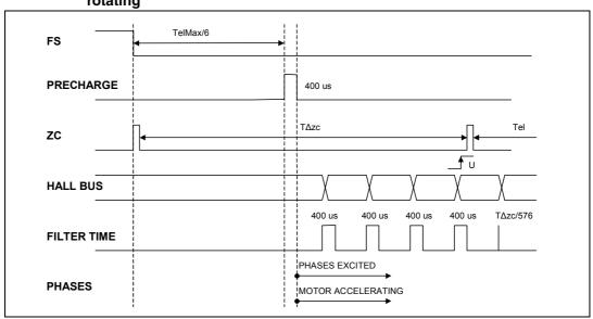
When the signal coming from the FS comparator has a falling edge (corresponding to a Vsp signal crossing the 1.23V threshold), the logic starts counting, to verify if the motor is rotating or not. If the motor is stopped and no Hall effect commutation is detected, the counter has reached its saturation time, given by the following equation:
