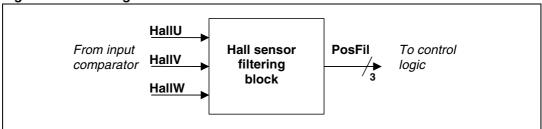
In order to simplify the explanation of the filtering circuit a signal Pos will be defined that can assume 7 different values according to the following table:
