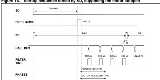
Startup sequence forced by SD, supposing the motor stopped
