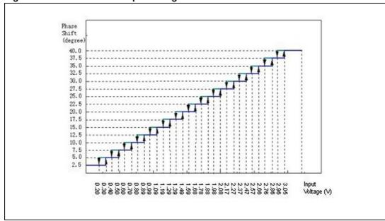
The 4-bit A/D has an internal hysteresis so that "Analog high thresholds" are the A/D thresholds applying a rising edge on TO pin, the "Analog low thresholds" are the A/D thresholds applying a falling edge on TO pin.
