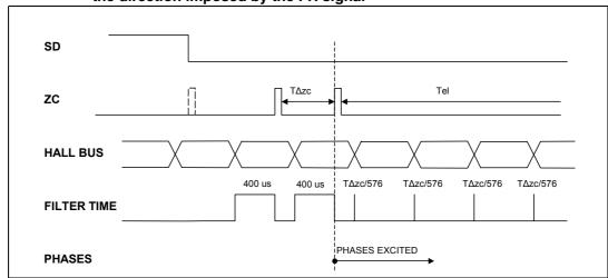
Startup sequence forced by SD, supposing the motor rotating quickly in Figure 19. the direction imposed by the FR signal
