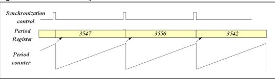
Figure 5. 16 bit counter operation
