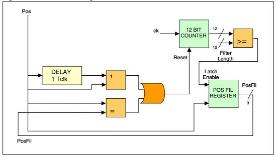
Figure 12. Filter Block Diagram
