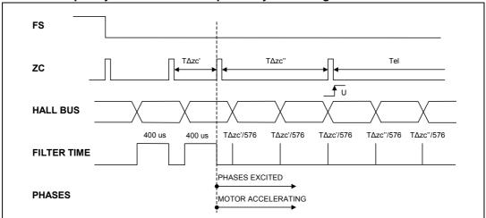
When the signal coming from the FS comparator has a falling edge, by default a zero-crossing signal is generated and the logic waits for a Hall effect commutation and applies to it a filtering time of  $T_{\mbox{\footnotesize{PRECHARGE}}}=400\mu\mbox{\footnotesize{\mu}sec}$ . The first significant zero-crossing signal is generated.
