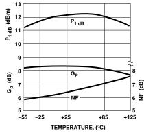
Figure 4. Output Power at 1 dB Gain Compression, NF and Power Gain vs. Case Temperature, f = 1.0 GHz,  $I_d = 50$  mA.
