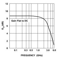
Figure 1. Typical Power Gain vs. Frequency,  $T_A = 25^{\circ}C$ ,  $I_d = 50$  mA.
