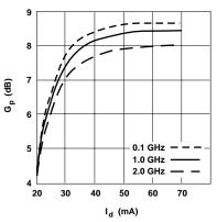
e. Figure 3. Power Gain vs. Current.
