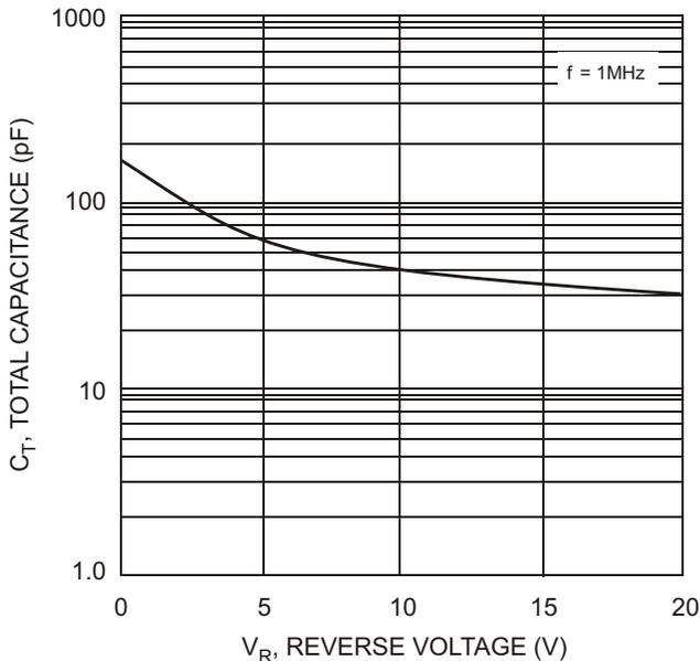
Fig. 5 Typ. Total Capacitance vs Reverse Voltage
