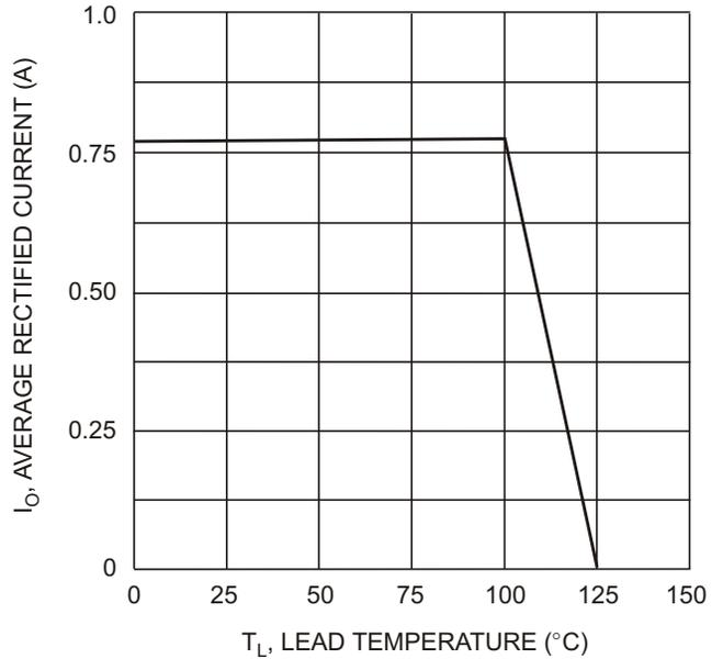
Fig. 2 Forward Current Derating
