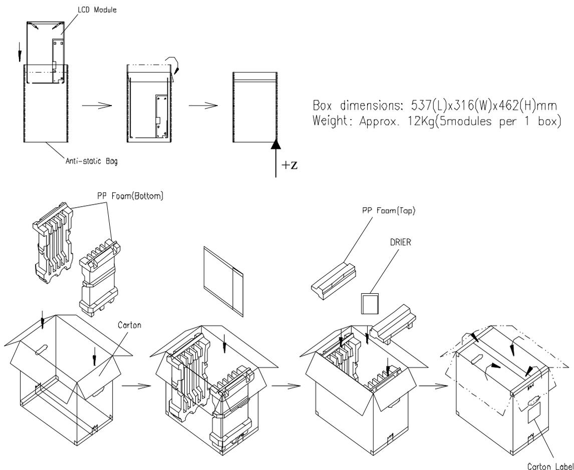
**Figure. 8-1 Packing method**
