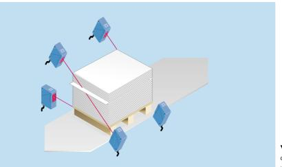
▼ A WT 260 photoelectric proximity switch controlling a commissioning system used in the wood-working industry.
