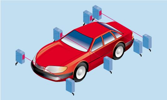
$\blacktriangle$  WS/WE 260 through-beam photoelectric switches used for detecting the outline of vehicle bodies on assembly lines in the automotive industry.
