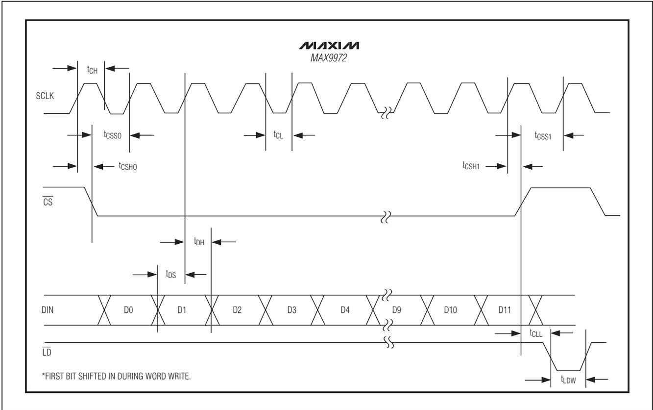
Figure 5. Serial-Interface Timing
