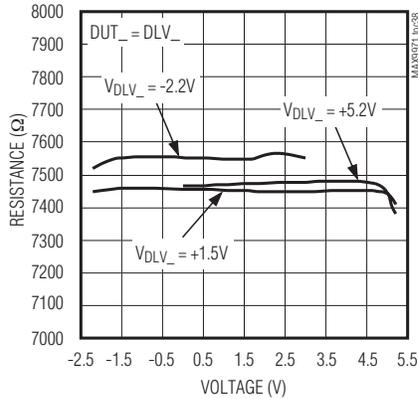
**PASSIVE LOAD LOW RESISTOR vs. VOLTAGE**
