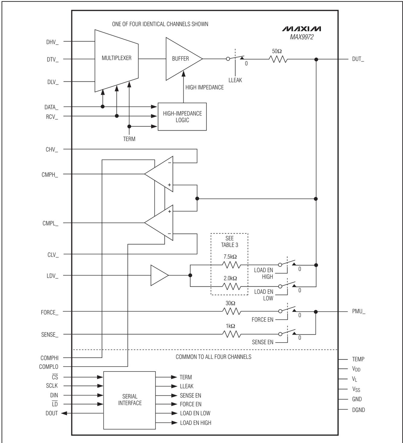
Figure 1. Block Diagram
