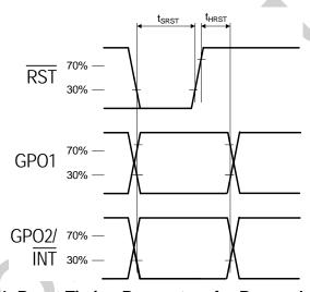
Figure 1. Reset Timing Parameters for Busmode Select
