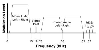
Figure 9. MPX Signal Spectrum
