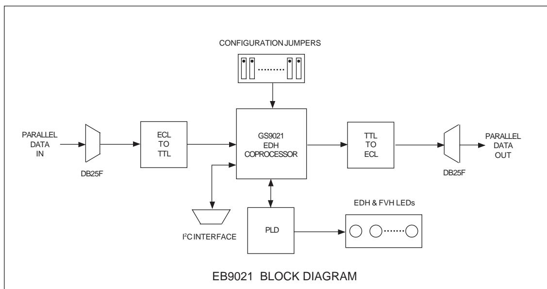
Finally, configuration jumpers are provided for further configuration of the GS9021. A detailed description of the input and output pins of the GS9021 can be found in the GS9021 data sheet.
