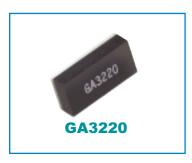
GA3220 is a system-in-a-package (SiP) signal processing platform specifically designed for hearing instruments which require high precision processing and ultra low power consumption. The platform delivers high-performance audio processing with superior power efficiency enabling the implementation of advanced
