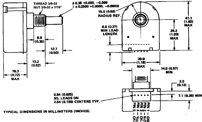
\*Note: For the HEDS-5700, Pin #2 is a No Connect. For the HEDS-5740, Pin #2 is Channel I, the index output.
