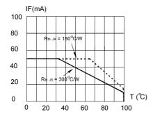
FIG.5 MAXIMUM FORWARD DC CURRENT VS TEMPERATURE. DERATING BASED ON Tjmax=110 Ĉ
