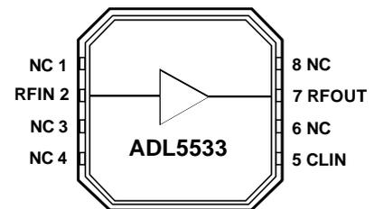
Figure 1. Block Diagram
