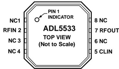
Figure 2. Pin Configuration
