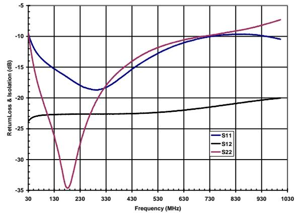
Figure 5 ADL5533 Input / Output Return Loss and Reverse Isolation vs Frequency
