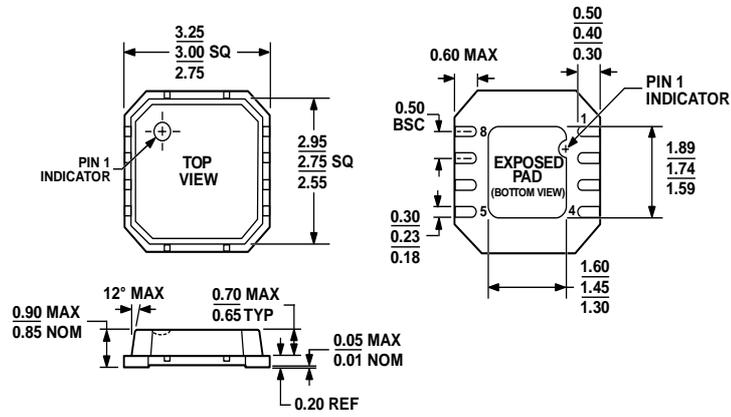
Figure 9. 8-Lead Lead Frame Chip Scale Package [LFCSP\_VD]
