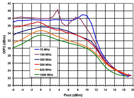
Figure 4 ADL5533 OIP3 vs Pout and Frequency
