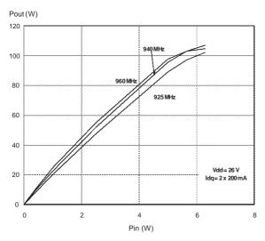
Output Power and Efficiency vs. Frequency
