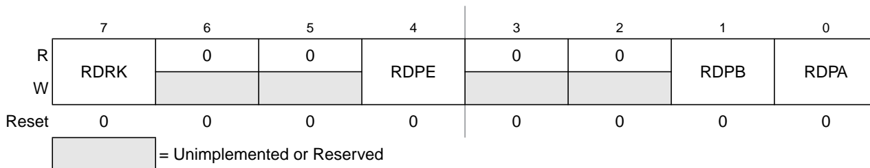
Figure 21-15. Reduced Drive Register (RDRIV)
