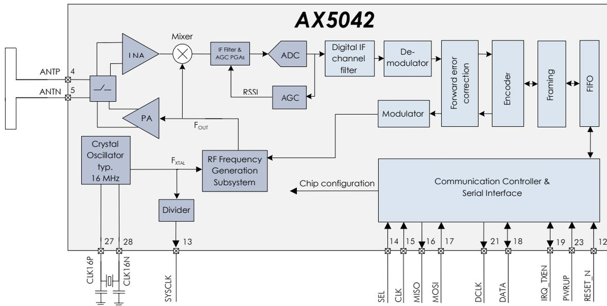
Figure 1 Functional block diagram of the AX5042
