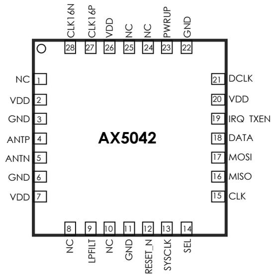
Figure 2: Pinout drawing (Top view)
