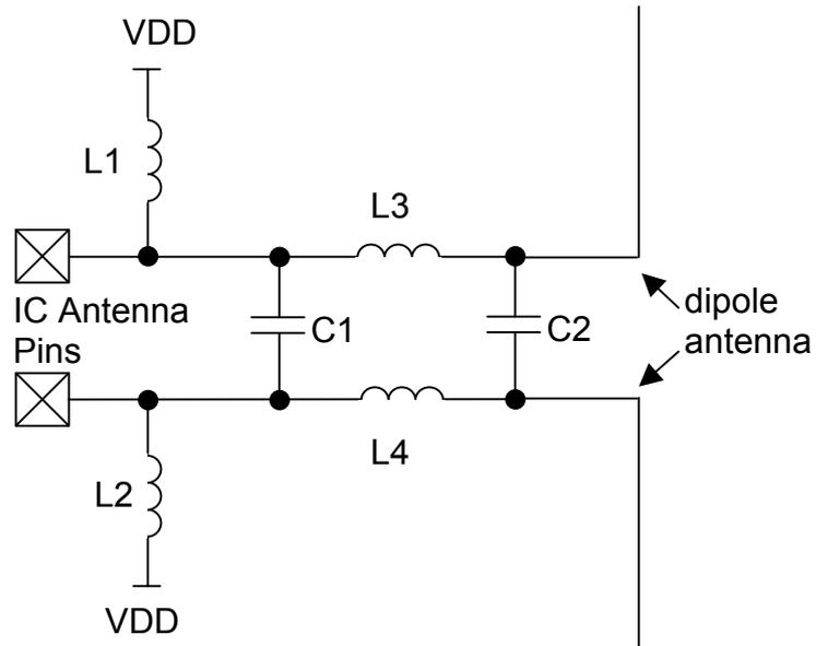
Figure 7 Structure of the antenna interface to a dipole antenna
