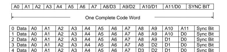
The Code Bits A0  $\sim$  A7 and A8/D3  $\sim$  A11/D0 are determined by the states of A0  $\sim$  A7 and A8/D3  $\sim$  A11/D0 pins. For example, when the A0 (Pin No. 1) is set to "1" (VCC), the Code Bit A0 is synthesized as "1" bit. In the same manner, when it (A0 Pin) is set to "0" (VSS) or left floating, the Code Bit A0 is synthesized as a "0" or "f" bit respectively.
