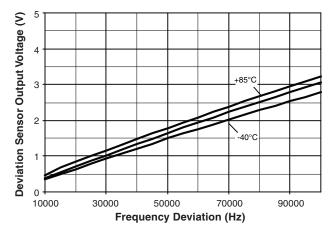
Note: FM modulation frequency: 1 kHz; BW setting 2<sup>nd</sup> IF filter = 120 kHz; demodulator fine tuning (bit 53 = 0)
