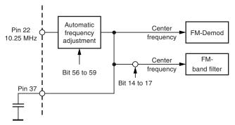
For fine tuning, the center frequency of all these integrated active filters (band filter and demodulator) can be shifted in steps of 6.25 kHz by means of bit 56 to bit 59. Additionally, the center frequency of the band filter can be adjusted separately by means of bit 14 to bit 17.
