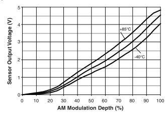
Note: AM modulation frequency 20 kHz; generator level 40 dBµV
