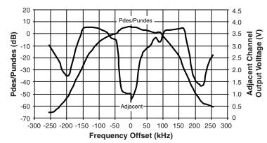
Note: Integrated bandfilter BW setting: 120 kHz Desired signal level adjusted to 40 dB S/N without undesired signal Undesired signal level adjusted to 26 dB S/N
