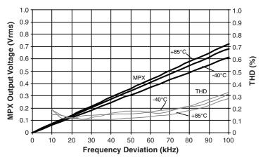
Note: Integrated band-filter BW setting: 120 kHz (bits 0 to 2 = 0, bit 3 = 1); 1 kHz modulation frequency; 50 µs de-emphasis (THD)
