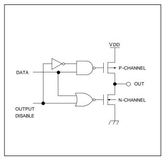
Figure 1-7. Pin Circuit Type C
