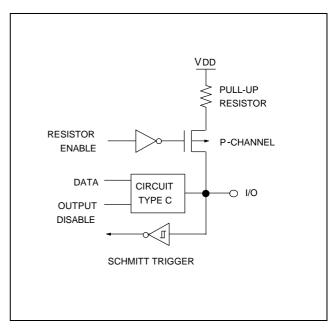
Figure 1-9. Pin Circuit Type D-1
