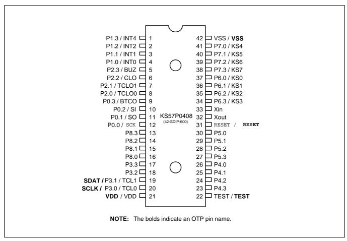
Figure 15–1. KS57P0408 Pin Assignments (42-SDIP Package)
