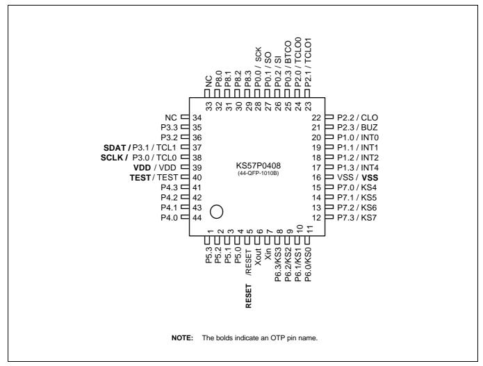
Figure 15-2. KS57P0408 Pin Assignments (44-QFP Package)
