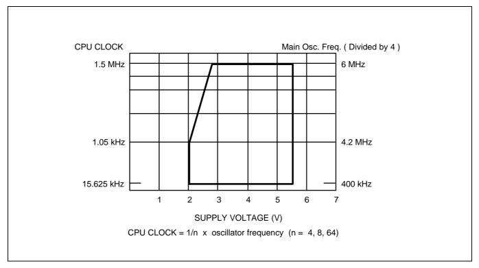
Figure 15-3. Standard Operating Voltage Range
