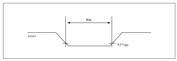
Figure 13-7. Input Timing for RESET Signal
