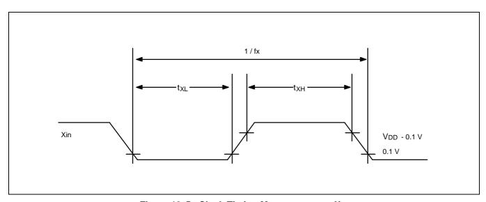
Figure 13–5. Clock Timing Measurement at Xin
