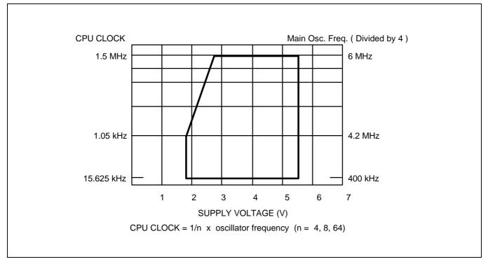
Figure 13-1. Standard Operating Voltage Range
