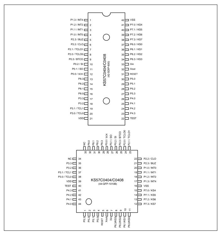
Figure 1-2. KS57C0404/C0408 Pin Assignment Diagrams
