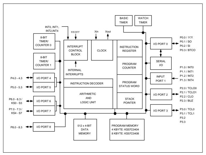
Figure 1-1. KS57C0404/C0408/P0408 Block Diagram
