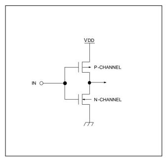
Figure 1-3. Pin Circuit Type A
