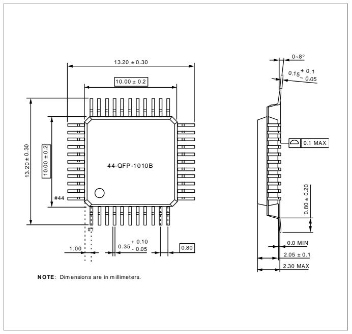
Figure 14–2. 44-QFP-1010B Package Dimensions
