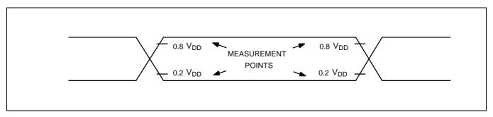
Figure 13–4. A.C. Timing Measurement Points (Except for Xin)
