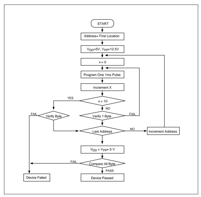
Figure 15-4. OTP Programming Algorithm
