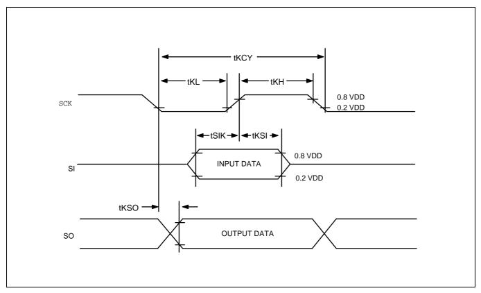
Figure 13-9. Serial Data Transfer Timing
