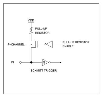
Figure 1-4. Pin Circuit Type A-3
