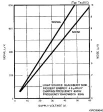
If a voltage higher than 60V is applied, the noise increases exponentially, degrading the S/N ratio The device should be operated at 60V or less
