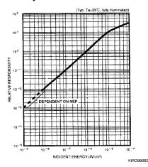
When making the incident light spot is smaller than the active area, the upper limit of the linearity becomes lower.
