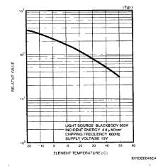
Cooling the device enhances its responsivity But the responsivity also depends on the load resistance in the circuit
