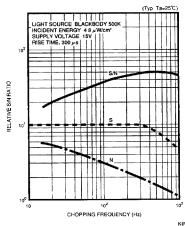
Increasing the chopping frequency reduces the 1/f noise and results in an improved S/N ratio. The S/N ratio can also be improved by narrowing the noise bandwidth using a lock-in amplifier.
