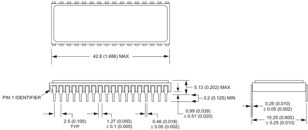
ALL LINEAR DIMENSIONS ARE MILLIMETERS AND PARENTHETICALLY IN INCHES
