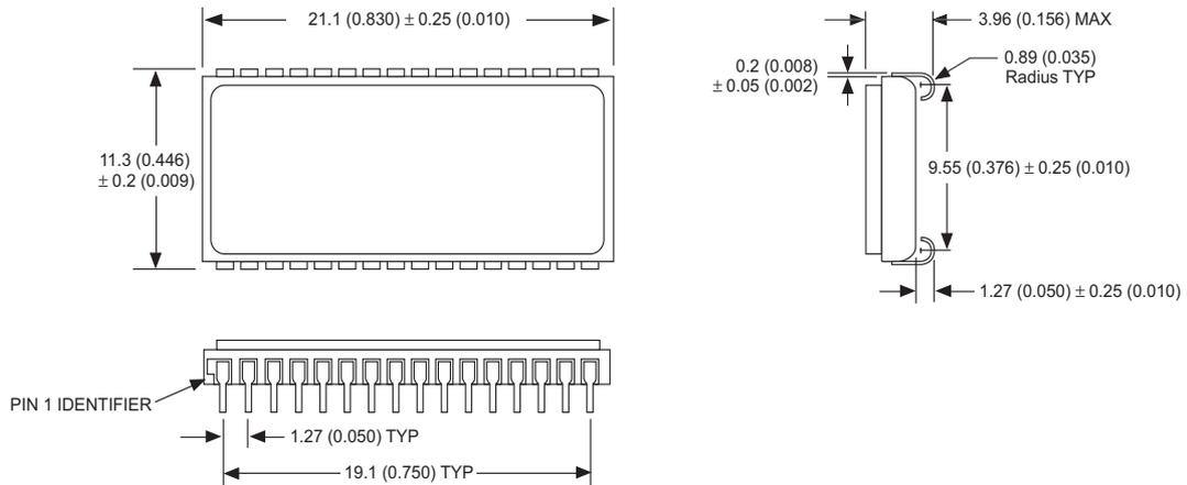
ALL LINEAR DIMENSIONS ARE MILLIMETERS AND PARENTHETICALLY IN INCHES
