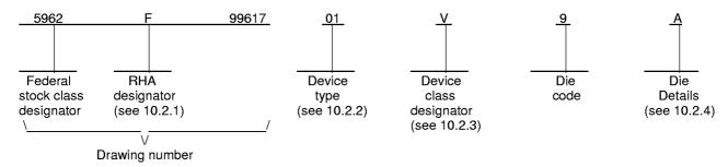
10.2.1 RHA designator. Device classes Q and V RHA identified die shall meet the MIL-PRF-38535 specified RHA levels. A dash (-) indicates a non-RHA die.
