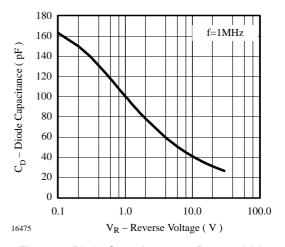
Figure 6. Diode Capacitance vs. Reverse Voltage
