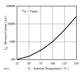
Figure 4. Reverse Current vs. Junction Temperature
