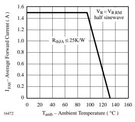
Figure 2. Max. Average Forward Current vs. Ambient Temperature
