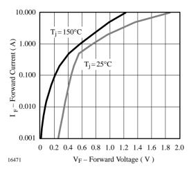
Figure 1. Forward Current vs. Forward Voltage
