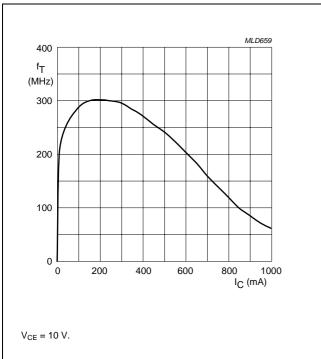
Fig.6 Transition frequency as a function of collector current; typical values.
