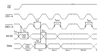
Note: (1) <u>A6</u> through A14 must specify the page address during each high to low transition of WE1~4 (or CS1~4). (2) OE must be high only when WE1~4 and CS1~4 are both low.
