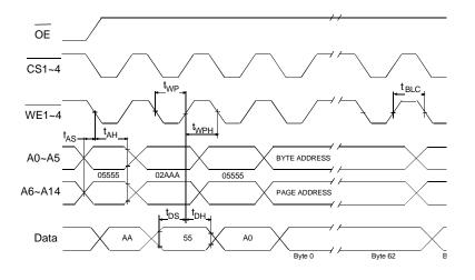
Notes: (1) A6 through A14 must specify the page address during each high to low transition of WE1~4 (or CS1~4). (2) OE must be high only when WE1~4 and CS1~4 are both low.
