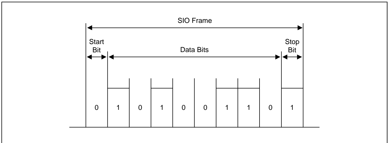
Figure 10-14. Serial I/O Frame Timing Diagram (Normal UART)
