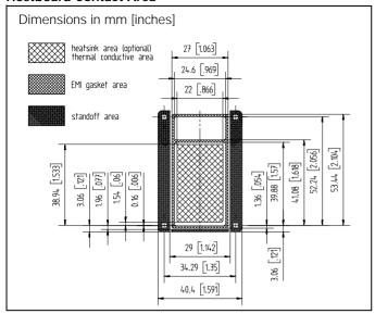
For the guaranteed EMI-performance an optimal electrical contact between the transponder housing and the user's pcb signal ground is necessary. For the user's pcb (hostboard) we recommend a full signal ground plane underneath the entire transponder housing (including the standoff area, the EMI gasket area and the optional heatsink area).
