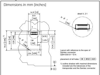
For detailed connector layout information, check http://www.samtec.com, and go to "QSH" connector.
