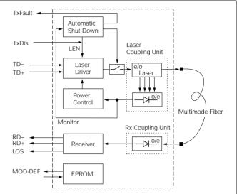
The receiver component converts the optical serial data into PECL compatible electrical data (RD and RDnot). The LOS of Signal (LOS, active low) shows whether an optical signal is present.
