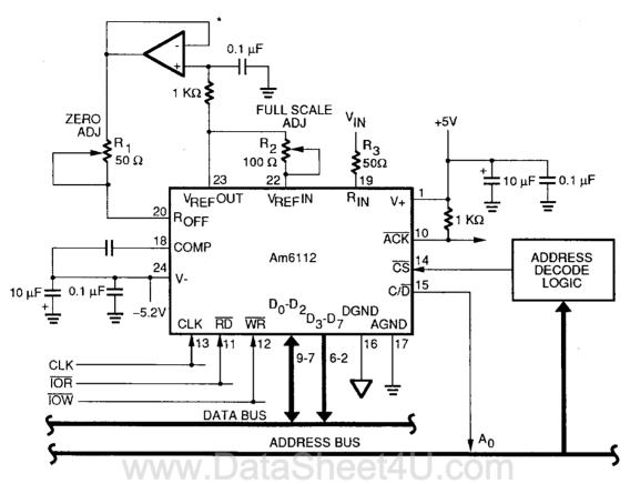
$^{\star}\text{A}$  low impedance Op Amp is recommended for optimum performance due to fast switching currents appearing at  $\text{R}_{\text{OFF}}$  .
