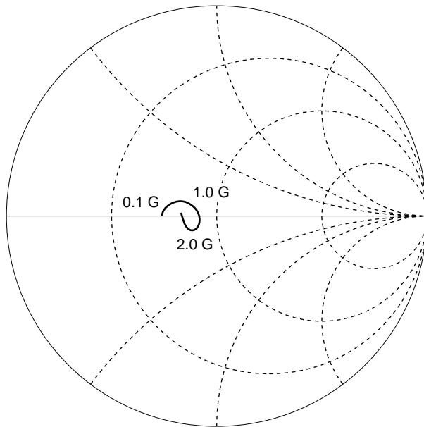
★ TYPICAL S-PARAMETER VALUES ( $T_A = +25^\circ\text{C}$ )–  $\mu$ PC2791TB – $V_{\text{CC}} = 5.0 \text{ V}$ ,  $I_{\text{CC}} = 17.0 \text{ mA}$
