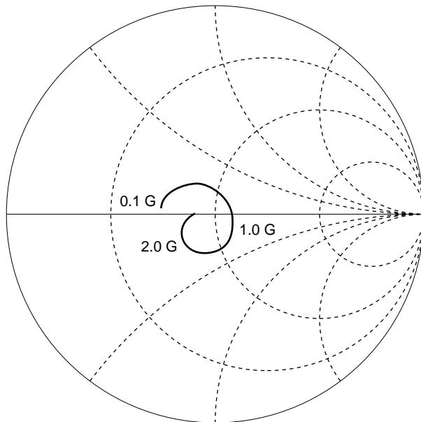
★ TYPICAL S-PARAMETER VALUES ( $T_A = +25^\circ\text{C}$ )–  $\mu$ PC2792TB – $V_{\text{CC}} = 5.0 \text{ V}$ ,  $I_{\text{CC}} = 19.0 \text{ mA}$
