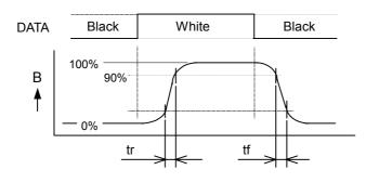
[Note 4] This shall be measured at center (point No.3 shown in Note 7).
