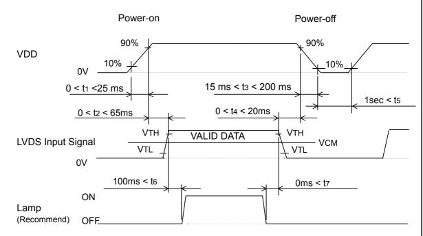
When the power is off, I/F Input Signal must be kept at either low level or high impedance.
