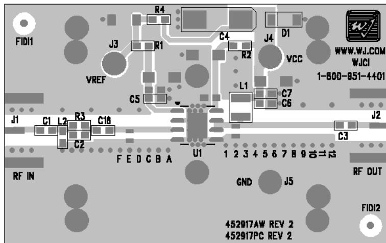
Circuit Board Material: .014" Getek, single layer, 1 oz copper, Microstrip line details: width = .026", spacing = .026" The silk screen markers 'A', 'B', 'C', etc. and '1', '2', '3', etc. are used as placemarkers for the input and output tuning shunt capacitors – C8 and C9. The markers and vias are spaced in .050" increments.
