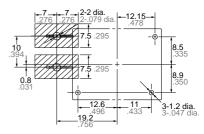
This product should only be used when there is no patterned metal surface (other than the terminal pattern) on the PC board facing the marked area
