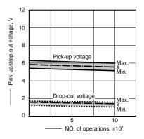
5-(2). Electrical life test Sample: JL1aZF-TMP1-12V, 5 pcs. Load: AC 125 V, 12 A Opetation frequency: 20 cpm (ON:OFF = 1.5s:1.5 s) Ambient temperature: 80°C 176°F
