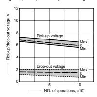
5-(3). Electrical life test Sample: JL1aGF-TMP1-12V, 5 pcs. Load: AC 125 V, 13 A Opetation frequency: 20 cpm (ON:OFF = 1.5 s:1.5 s) Ambient temperature : 90°C 194°F
