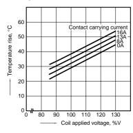
3. Ambient temperature characteristics (Contact carrying current: 16 A) Sample: JL1aGF-TMP1-12V, 6 pcs.
