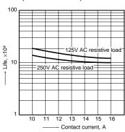
5-(1). Electrical life test Sample: JL1aGF-TMP1-12V, 6 pcs. Load: AC 277 V, 16 A, resistive load Opetation frequency: 20 cpm (ON:OFF = 1.5 s:1.5 s) Ambient temperature : 26°C 79°F circuit:
