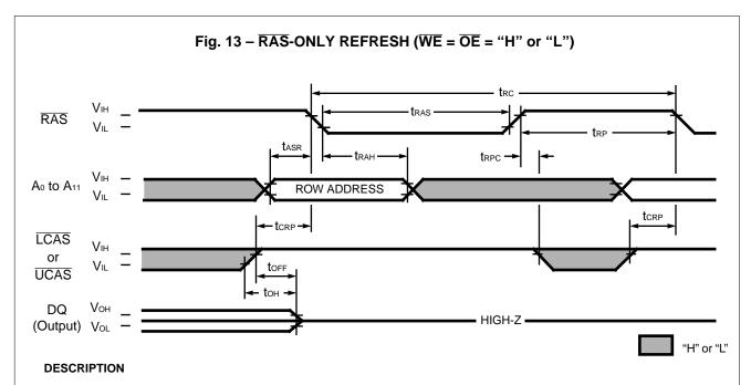
Refresh of RAM memory cells is accomplished by performing a read, a write, or a read-modify-write cycle at each of 4096 row addresses every 65.6-milliseconds. Three refresh modes are available: RAS-only refresh, CAS-before-RAS refresh, and hidden refresh.
