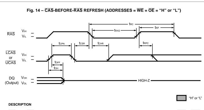
CAS-before-RAS refresh is an on-chip refresh capability that eliminates the need for external refresh addresses. If LCAS or UCAS is held Low for the specified setup time (tcsr) before RAS goes Low, the on-chip refresh control clock generators and refresh address counter are enabled. An internal refresh operation automatically occurs and the refresh address counter is internally incremented in preparation for the next CAS-before-RAS refresh operation.
