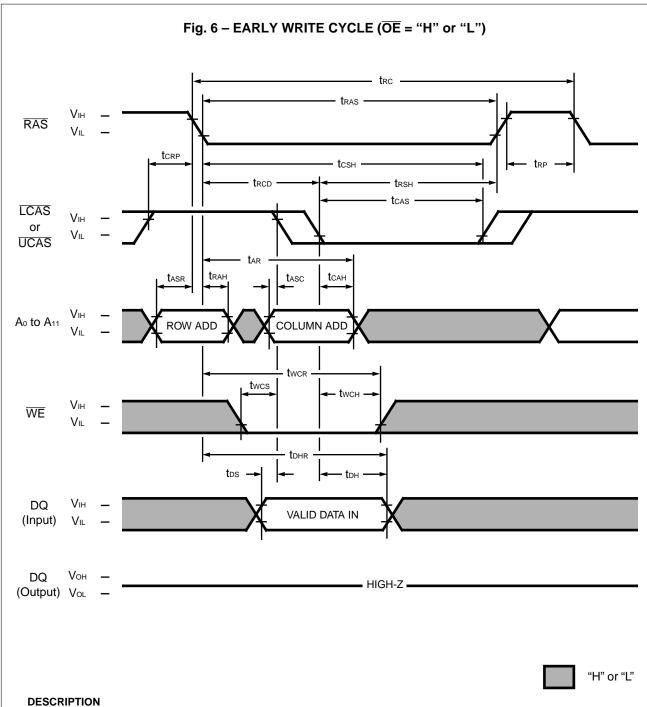
A write cycle is similar to a read cycle except WE is set to a Low state and  $\overline{\text{OE}}$  is an "H" or "L" signal. A write cycle can be implemented in either of three ways - early write, delayed write, or read-modify-write. During all write cycles, timing parameters truck, towk, tral and toal must be satisfied. In the early write cycle shown above two satisfied, data on the DQ pins are latched with the falling edge of LCAS or UCAS and written into memory.
