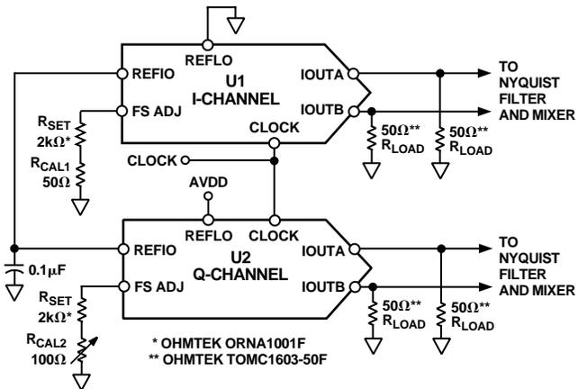
Figure 38. Baseband QAM Implementation Using Two AD9752s
