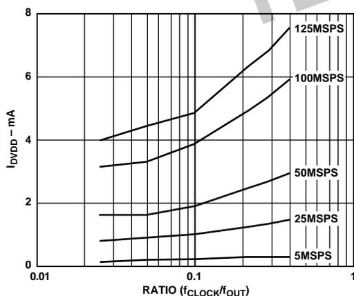
Figure 30.  $I_{DVDD}$  vs. Ratio @  $DVDD = 3\text{ V}$
