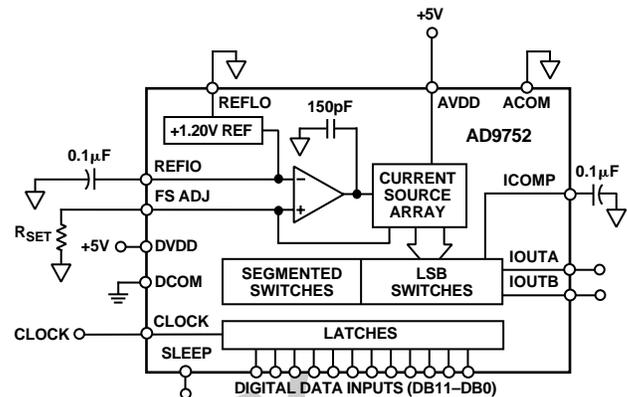
Differential current outputs are provided to support single-ended or differential applications. Matching between the two current outputs ensures enhanced dynamic performance in a differential output configuration. The current outputs may be tied directly to an output resistor to provide two complementary, single-ended voltage outputs or fed directly into a transformer. The output voltage compliance range is 1.25 V.
