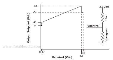
An open circuit on this pin reverts the voltage level back to the original setting.
