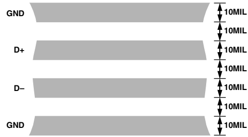
Figure 4. Arrangement of Signal Tracks
