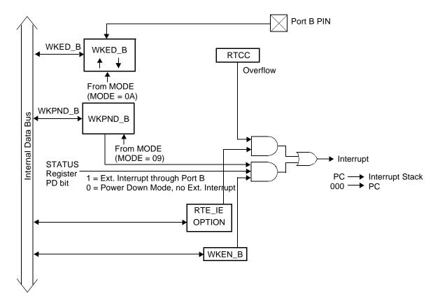
Figure 8-1. Interrupt Structure
