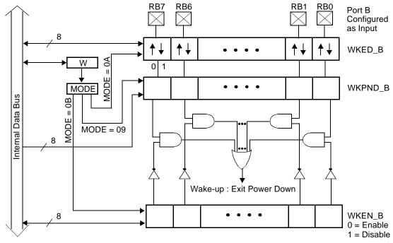
Figure 7-1. Multi-Input Wakeup Block Diagram
