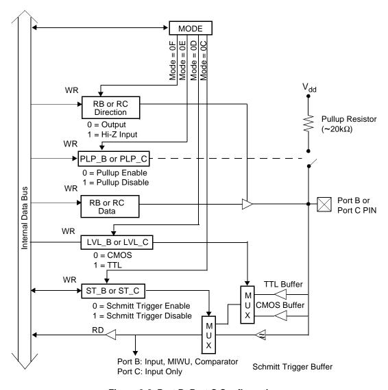
Figure 3-2. Port B, Port C Configuration
