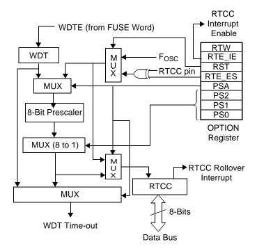
Figure 10-1. RTCC and WDT Block Diagram
