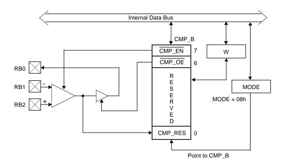
Figure 11-1. Comparator Block Diagram
