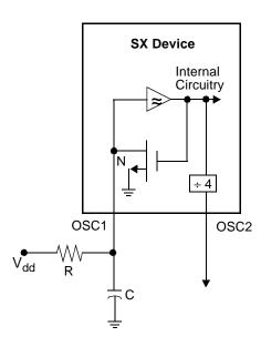
Figure 9-3. RC Oscillator Mode
