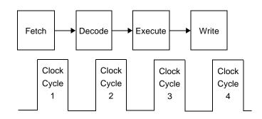
Figure 15-1. Pipeline and Clock Scheme
