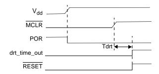
Figure 12-2. <u>Time-Out Sequence on Power-Up</u> (MCLR not tied to V<sub>dd</sub>)
