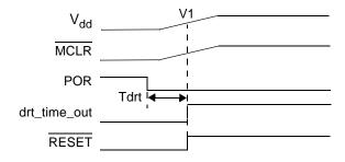
Figure 12-4. Time-out Sequence on Power-up (MCLR tied to V<sub>dd</sub>): Slow Rise Time
