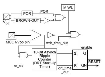
Note:Ripple counter is 10 bits for Power on Reset (POR) only.
