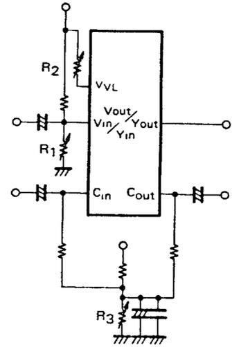
**Note:** Since there is no built-in pedestal clamp circuit for external video signal, connect direct current clamp circuit in front of "video in/Y in".
