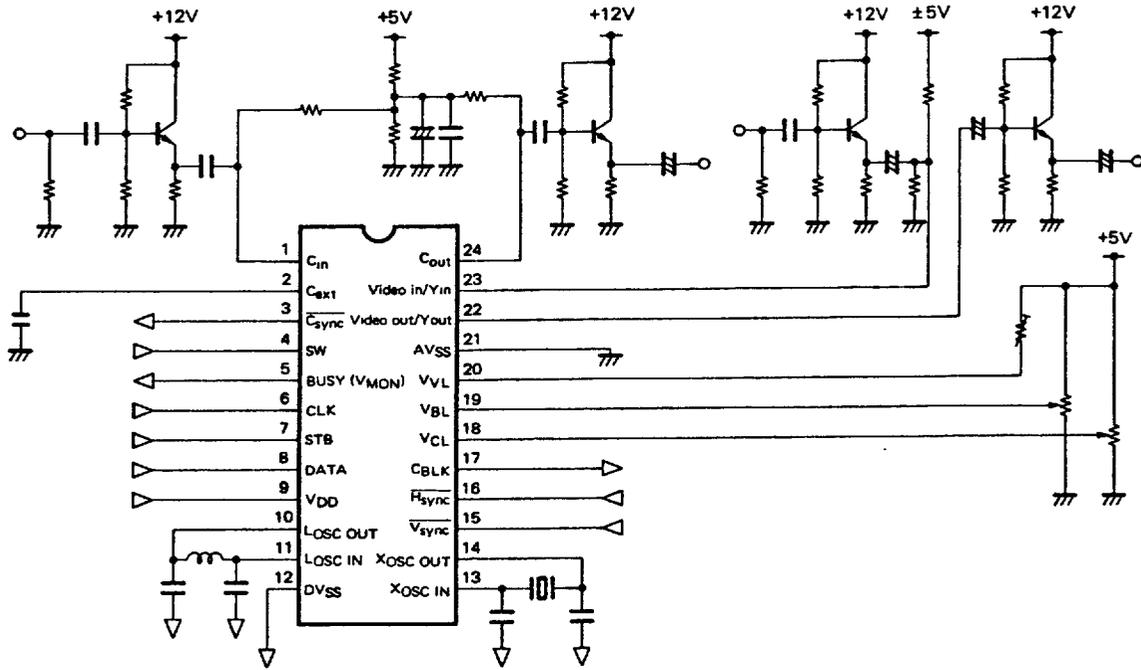
Note: The peripheral amplifier uses +12 V. To use +5 V, give attention to the amplifier configuration. Use analog ground  $\text{⏏}$  and digital ground  $\text{⏏}$  separate.
