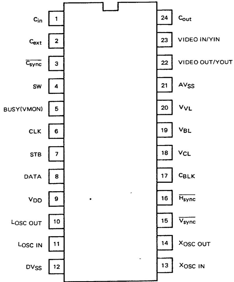
**Note:** This bracket shows terminal arrangement for the mask code option when terminal 5 of  $\mu$ PD6452 is used for the synchronization protection monitor output (VMON)
