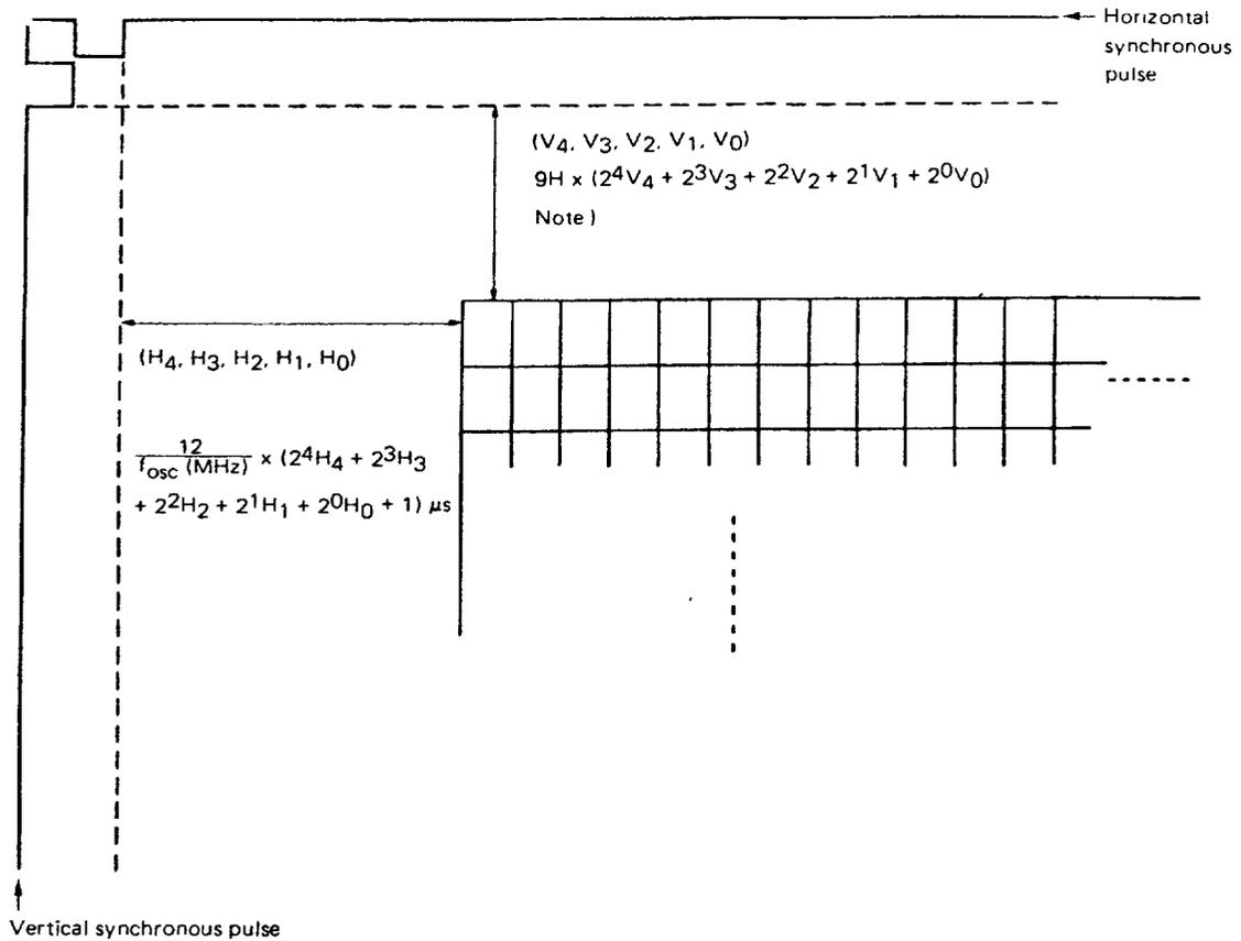
**Note:** Vertical address counter is incremented by the leading edge of the horizontal synchronous pulse.
