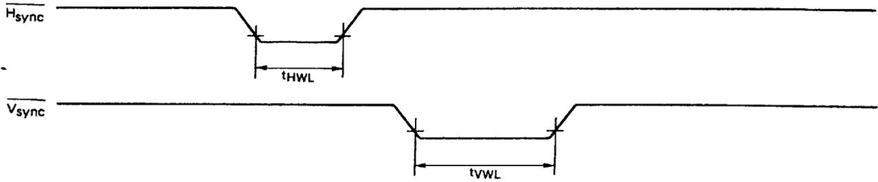
RECOMMENDED OPERATION TIMING ( $T_a = 25^\circ C, V_{DD} - V_{SS} = 5.0 V$ )
