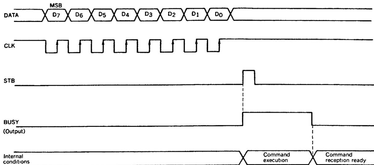
For format data, a busy signal is generated after the internal conditions are completely determined. When writing data in VRAM, a busy signal is generated after the completion of writing in VRAM. When the VRAM write period extends into the horizontal retrace line period, the busy signal becomes longer than usual, so be careful. (This is because oscillation is suspended during the horizontal retrace line period, so writing in VRAM becomes impossible.)
