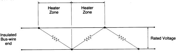
Rated Voltage - 220V/240V or 110V/120V AC/DC. Heater Zone (according to design) - 0.5/1.0m.
