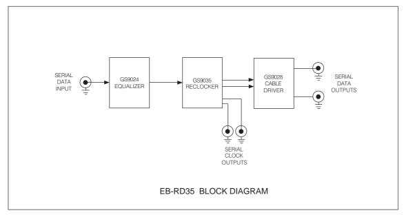
The CD\_ADJ input of the GS9024 is biased via a resistor network including a potentiometer allowing the user to adjust the level at which loss of carrier is detected. For a detailed description of the CD\_ADJ voltage level versus muting threshold refer to the GS9024 data sheet. Turning the potentiometer completely clockwise allows for maximum possible cable length equalization. In addition, the GS9024 outputs can be put in a HIGH-Z state by putting jumper JMP1 into the 1-2 position.
