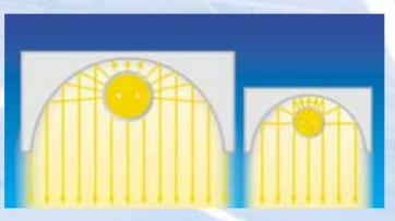
Slim lamp, compact reflector: With the lamp diameter reduced to 16 mm the reflectors can be 40% smaller for the same shading.
