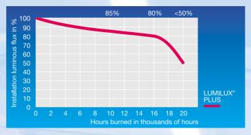
The small drop in installation luminous flux is thanks to the new LUMILUX® PLUS phosphor which increases the service life (mortality x maintenance)
