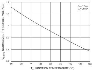
Fig. 3 Gate Threshold Variation with Temperature
