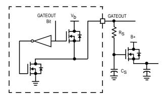
Figure 11. External N-FET Gate Drive Circuit
