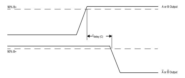
Figure 5. Step Motor Crossover Delay Timing
