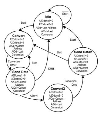
Note "Start" is bit 1 of the serial input normal frame.
