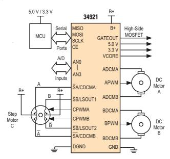
Figure 1. 34921 Simplified Application Diagram
