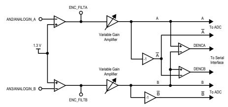
Figure 13. Analog Encoder Interface Block Diagram
