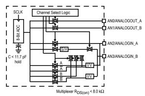
Figure 14. A/D Converter Input Structure
