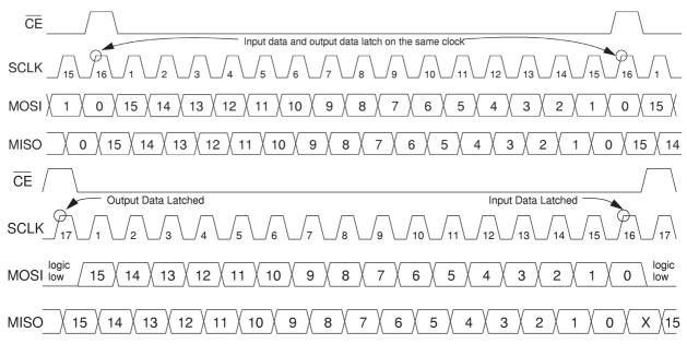
Figure 4. Serial Interface Timing
