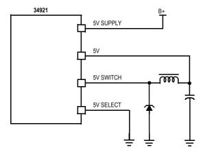
Figure 8. 5.0 V Switching Regulator Mode
