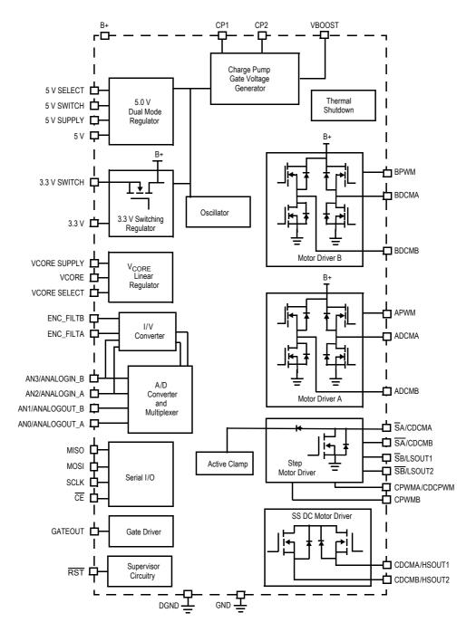
Figure 2. 34921 Simplified Internal Block Diagram
