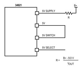
Figure 9. 5.0 V Linear Regulator Mode
