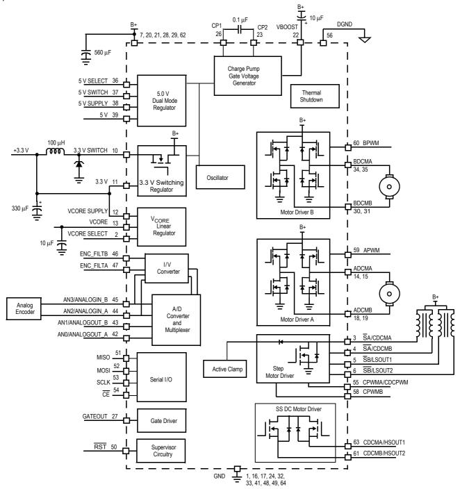
Figure 15. TYPICAL APPLICATION DIAGRAM
