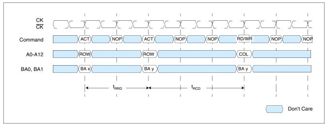
Figure 8  $t_{RCD}$  and  $t_{RRD}$  Definition
