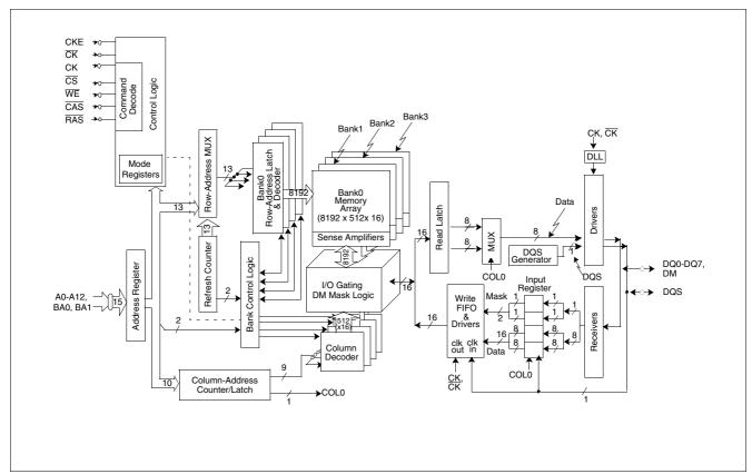
Figure 4 Block Diagram (32Mb × 8)
