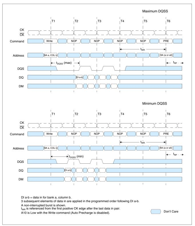
Figure 26 Write to Precharge: Non-Interrupting (Burst Length = 4)
