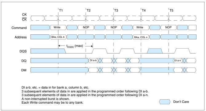
Figure 20 Write to Write: Max. DQSS, Non-Consecutive (Burst Length = 4)
