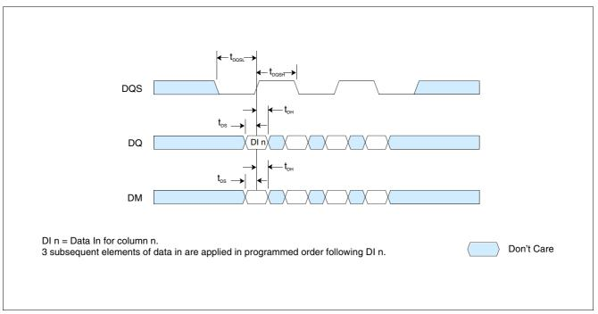
Figure 38 Data Input (Write), Timing Burst Length = 4
