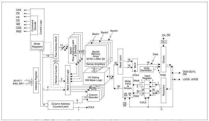
Figure 5 Block Diagram (16Mb × 16)
