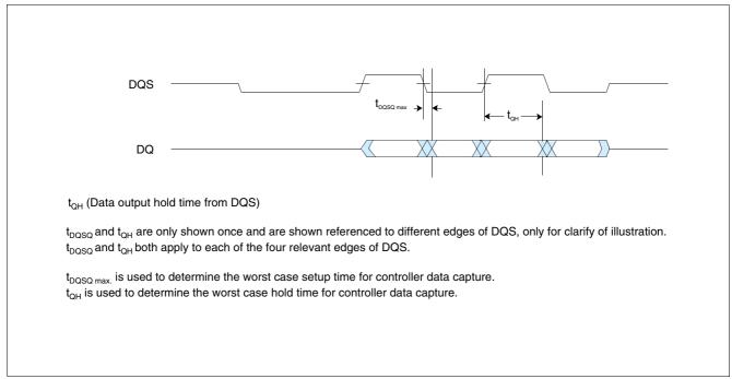
Figure 39 Data Output (Read), Timing Burst Length = 4
