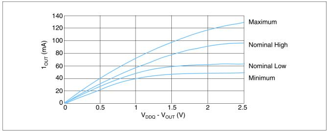
Figure 33 Normal Strength Pull-down Characteristics
