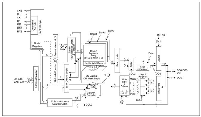
Figure 3 Block Diagram (64Mb × 4)
