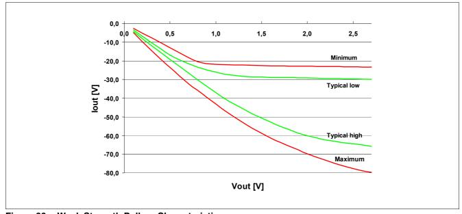
Figure 36 Weak Strength Pull-up Characteristics
