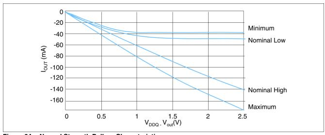
Figure 34 Normal Strength Pull-up Characteristics
