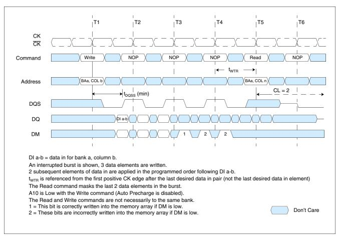
Figure 24 Write to Read: Minimum DQSS, Odd Number of Data (3-bit Write), Interrupting (CAS Latency = 2; Burst Length = 8)
