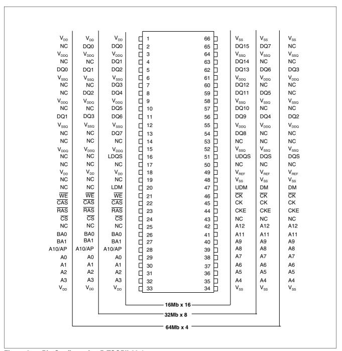
Figure 2 Pin Configuration P-TSOPII-66-1
