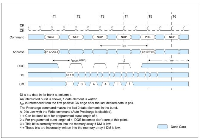
Figure 28 Write to Precharge: Minimum DQSS, Odd Number of Data (1-bit Write), Interrupting (Burst Length = 4 or 8)
