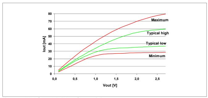
Figure 35 Weak Strength Pull-down Characteristics
