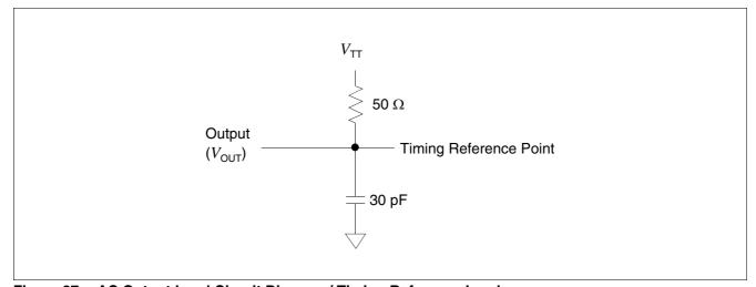
Figure 37 AC Output Load Circuit Diagram / Timing Reference Load
