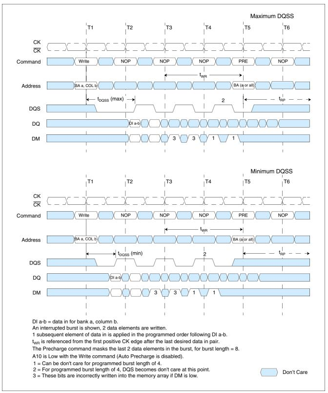
Figure 27 Write to Precharge: Interrupting (Burst Length = 4 or 8)
