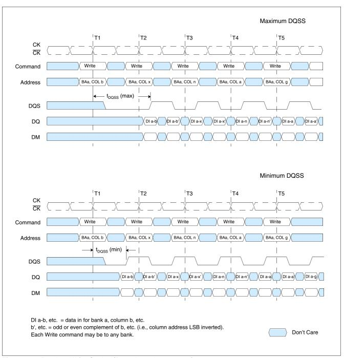
Figure 21 Random Write Cycles (Burst Length = 2, 4 or 8)
