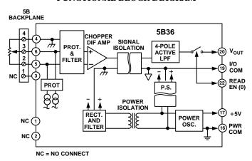
at 50 Hz. Output noise is an exceptionally low 0.3 mV p-p at 100 kHz bandwidth and 6 mV p-p at 5 MHz bandwidth.
