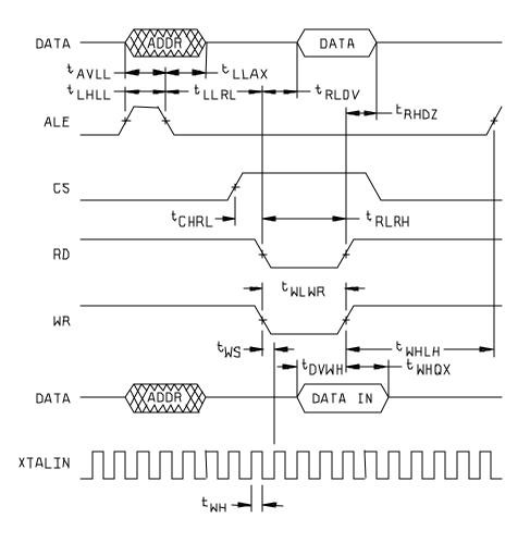
FIGURE 4. Timing waveforms.
