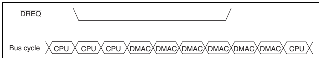
Figure 9.8 DMA Transfer Example in the Burst Mode
