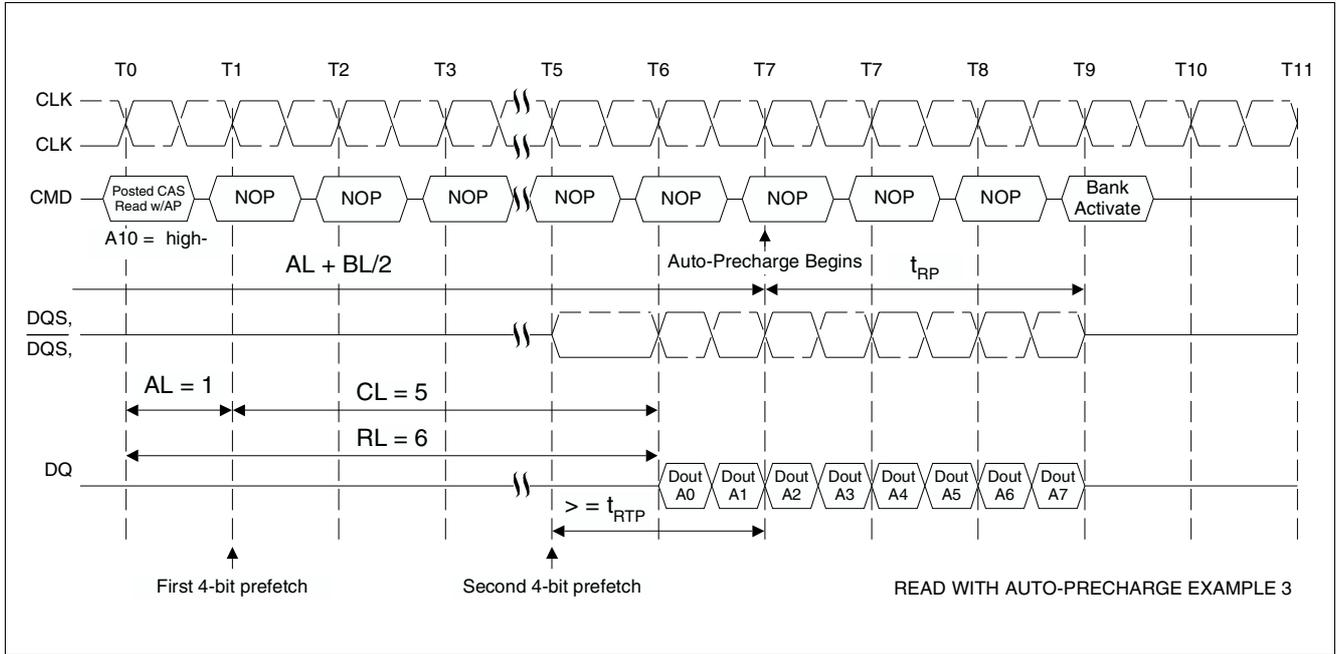
**Figure 43** Read with Auto-Precharge Example 3, followed by an Activation to the Same Bank:
