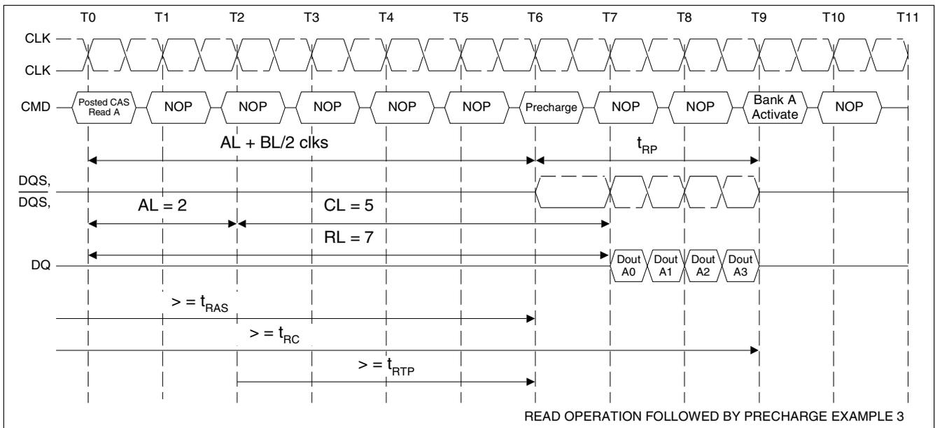
**Figure 37 Read Operation Followed by Precharge Example 3:**
