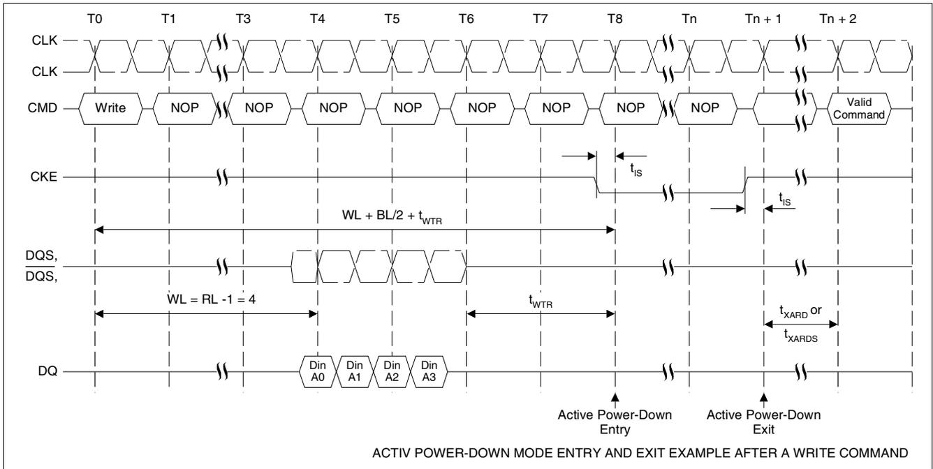
**Figure 50 Active Power-Down Mode Entry and Exit Example after a Write Command:**
