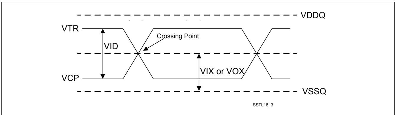
Figure 58 Differential DC and AC Input and Output Logic Levels Diagram
