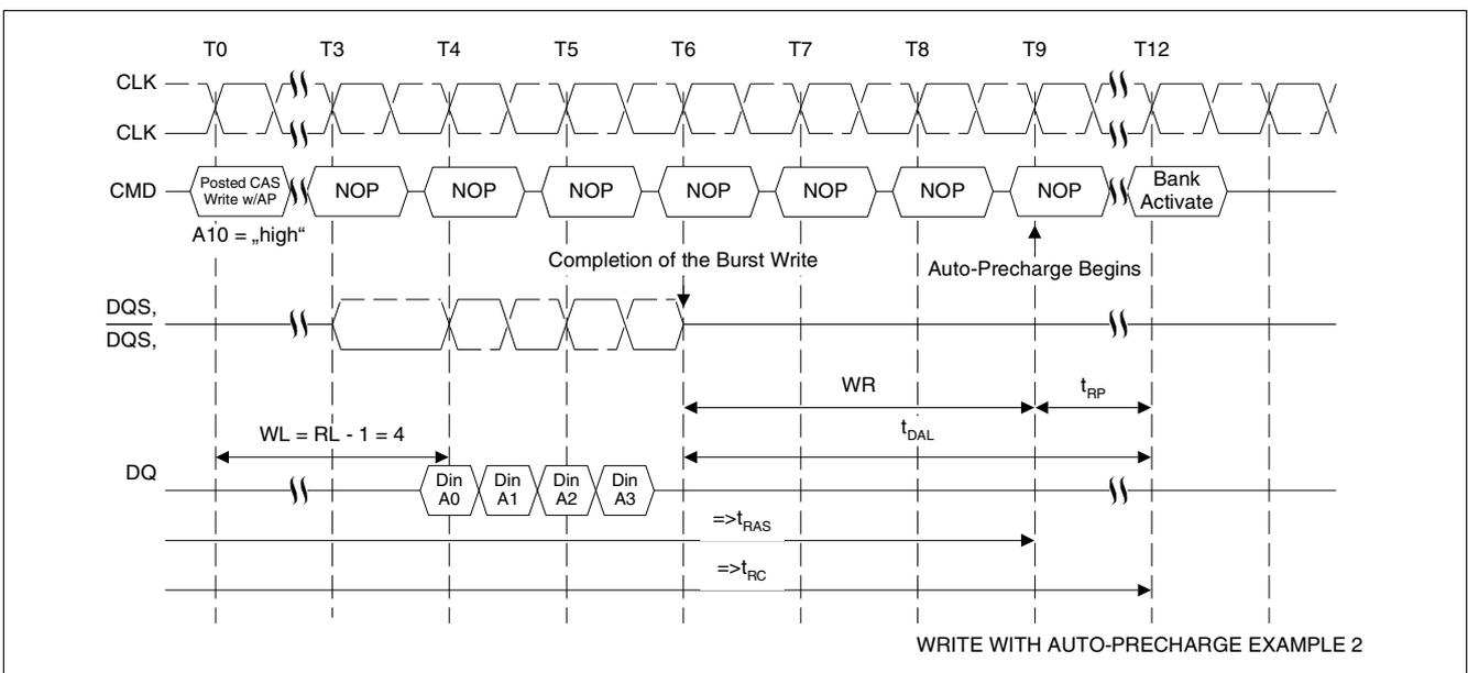
Figure 45 Write with Auto-Precharge Example 2 ( $WR + t_{RP}$  Limit):  $WL = 4$ ,  $t_{DAL} = 6$  ( $WR = 3$ ,  $t_{RP} = 3$ ),  $BL = 4$
