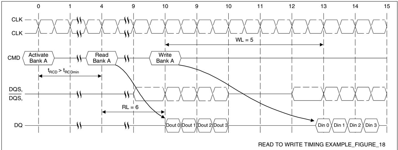
**Figure 18 Read to Write Timing Example: Read followed by a write to the same bank, Activate to Read delay >  $t_{RCDmin}$ : AL = 1, CL = 5, RL = 6, WL = 5, BL = 4**
