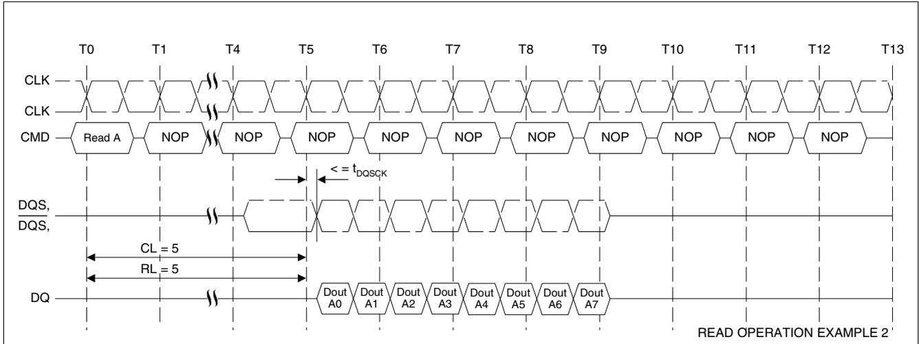
Figure 21 Read Operation Example 2:  $RL = 5$  ( $AL = 0$ ,  $CL = 5$ ,  $BL = 8$ )
