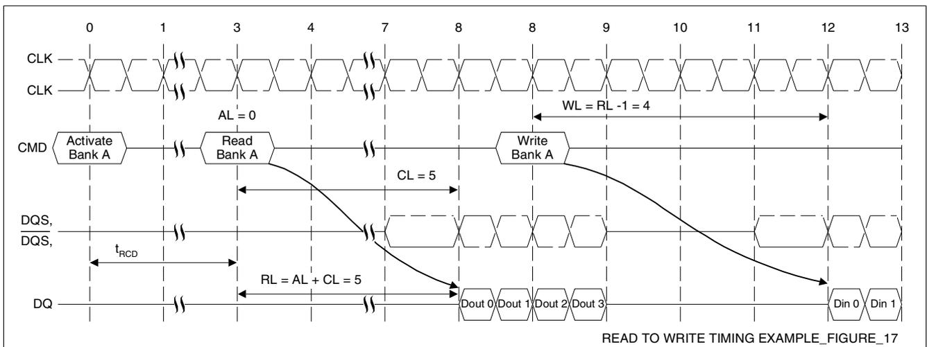
**Figure 17 Read to Write Timing Example: Read followed by a write to the same bank, Activate to Read delay =  $t_{RCDmin}$ : AL = 0, CL = 5, RL = (AL + CL) = 5, WL = (RL - 1) = 4, BL = 4**
