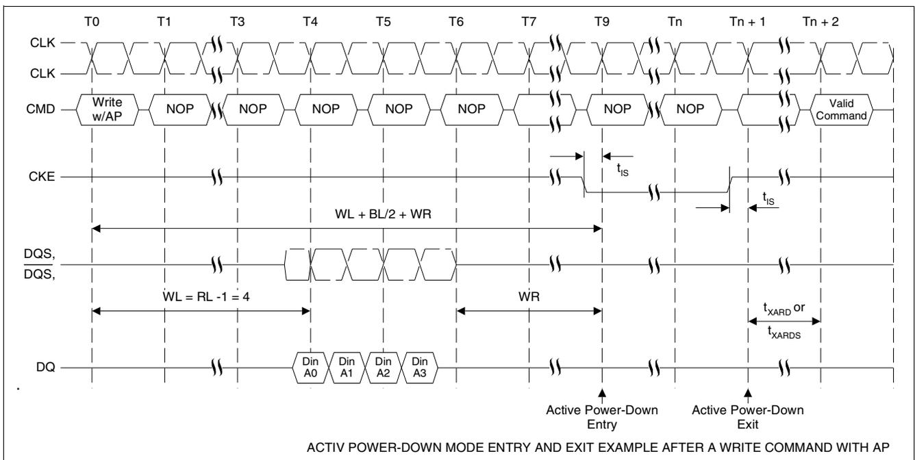
**Figure 51 Active Power-Down Mode Entry and Exit Example after a Write Command with AP:**
