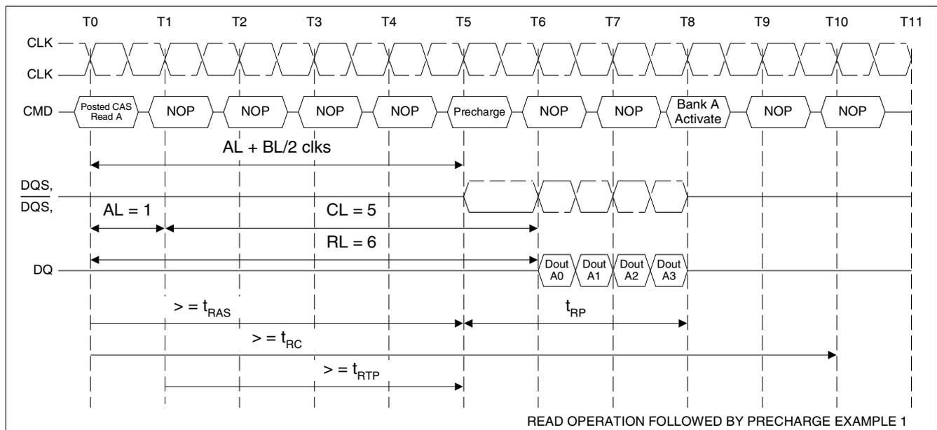
**Figure 35 Read Operation Followed by Precharge Example 1:**
