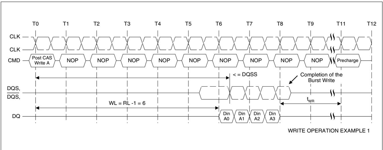
Figure 26 Write Operation Example 1: RL = 7 (AL = 2, CL = 5), WL = 4, BL = 4
