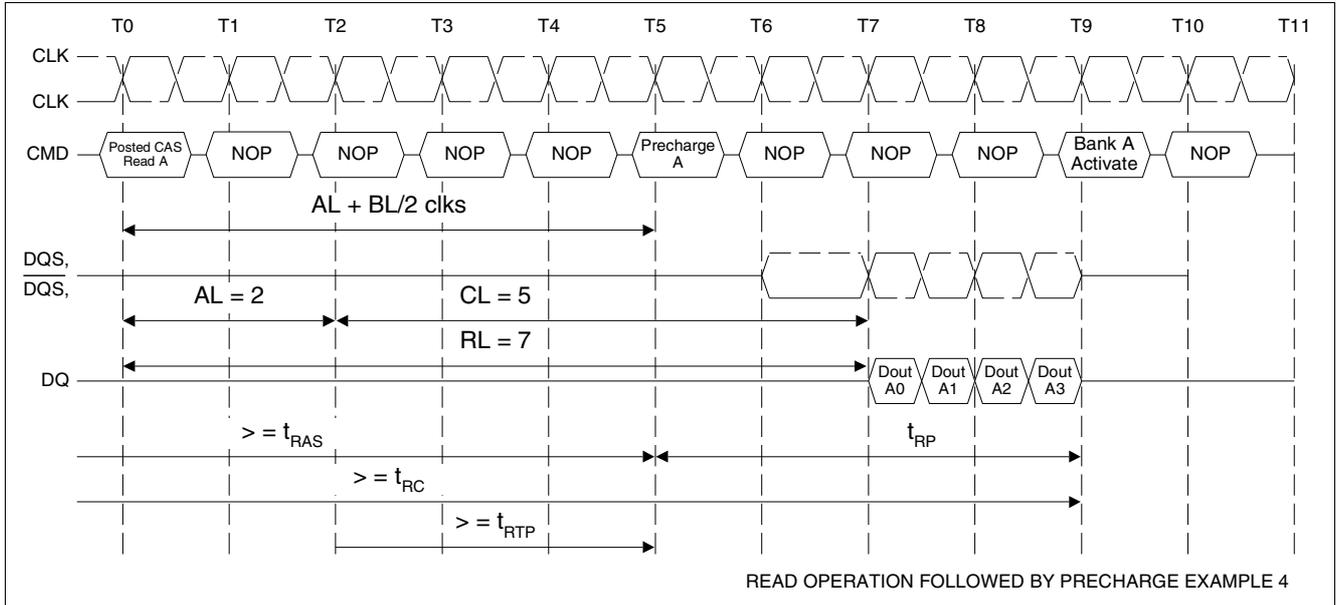
**Figure 38 Read Operation Followed by Precharge Example 4:**
