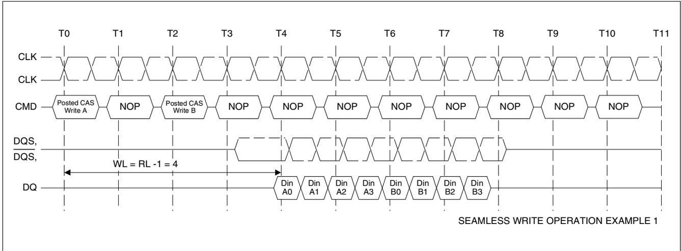
**Figure 29 Seamless Write Operation Example 1: RL = 5, WL = 4, BL = 4**
