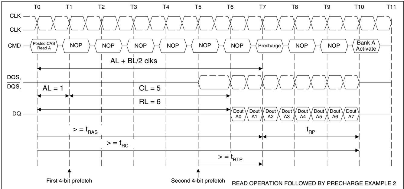
**Figure 36 Read Operation Followed by Precharge Example 2:**
