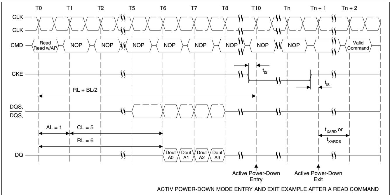
**Figure 49 Active Power-Down Mode Entry and Exit Example after a Read Command:
