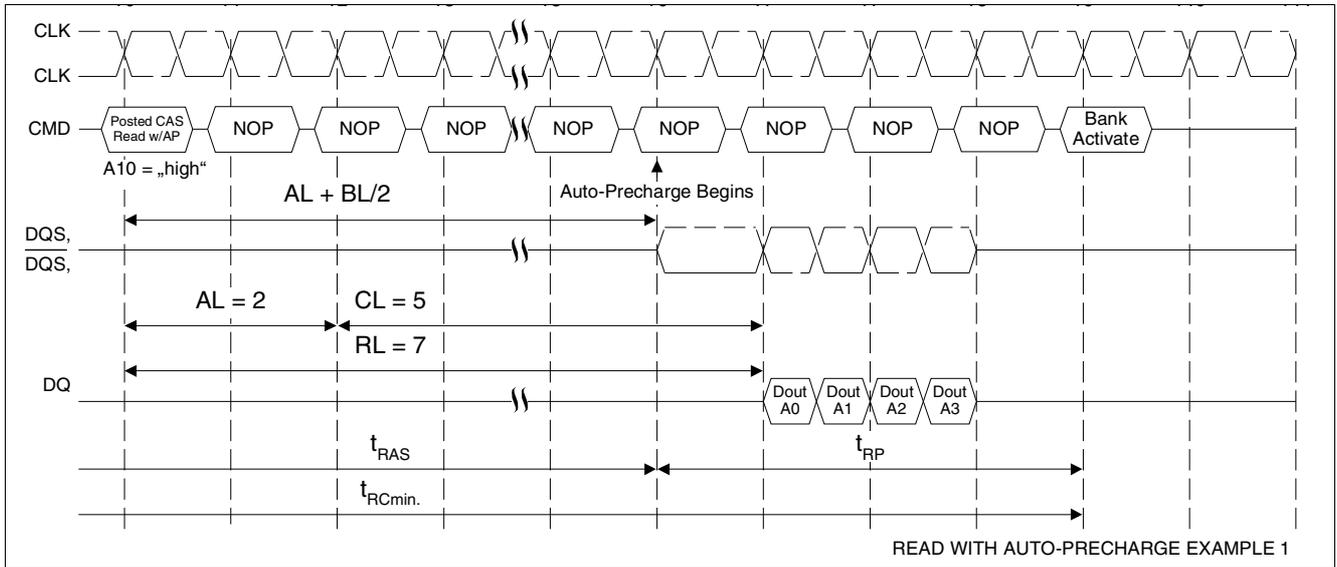
**Figure 41** Read with Auto-Precharge Example 1, followed by an Activation to the Same Bank ( $t_{RC}$  Limit):
