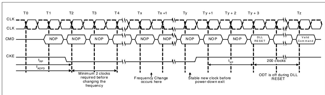
Figure 55 Input Frequency Change Example during Precharge Power-Down mode
