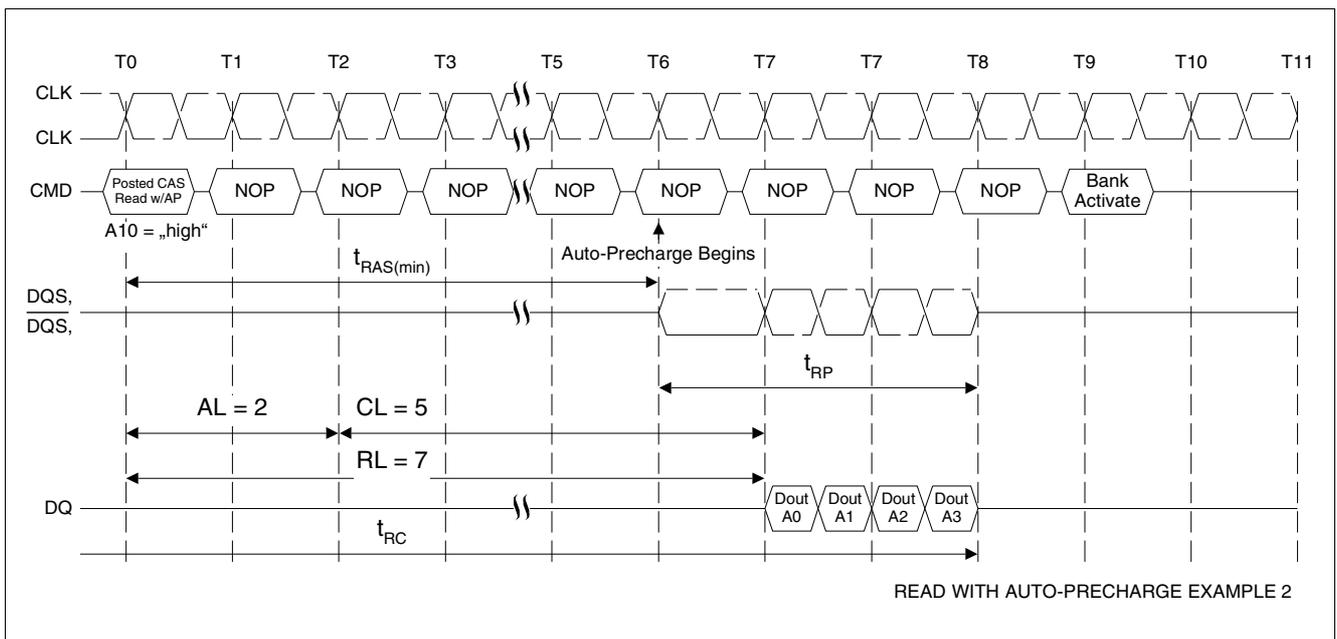
**Figure 42** Read with Auto-Precharge Example 2, followed by an Activation to the Same Bank ( $t_{RAS}$  Limit):
