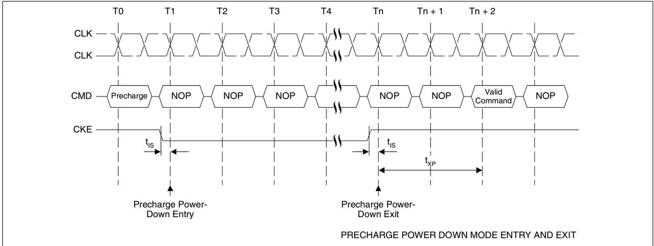
Figure 52 Precharge Power Down Mode Entry and Exit
