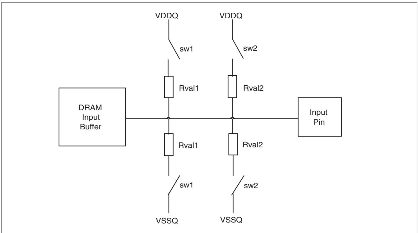
**Figure 8 Functional Representation of ODT**
