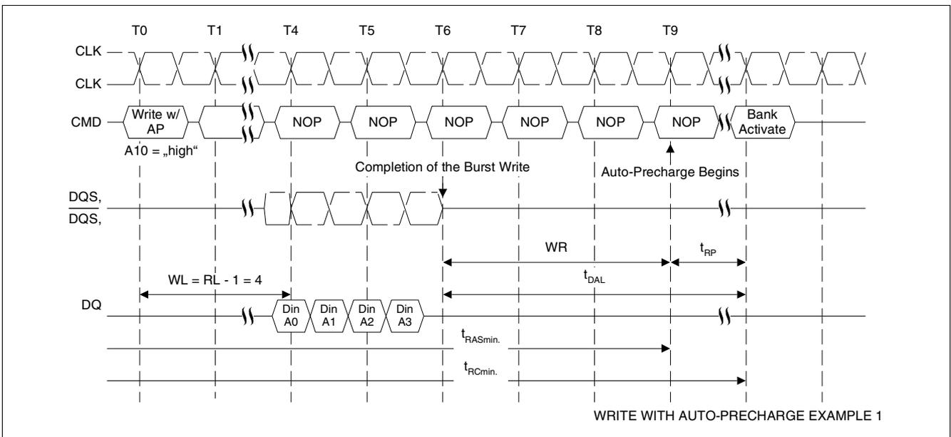
Figure 44 Write with Auto-Precharge Example 1 ( $t_{RC}$  Limit):  $WL = 4$ ,  $t_{DAL} = 6$  ( $WR = 3$ ,  $t_{RP} = 3$ ),  $BL = 4$
